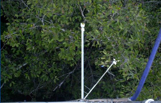
Three surface wetness logging sensors are installed offset from the towers at three heights: canopy top (32 m), canopy base (25 m) near the forest floor (3m)
