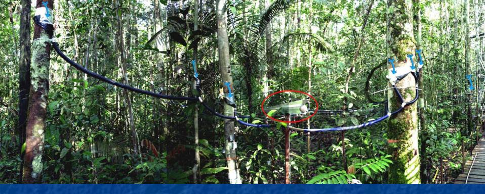
Stemflow is collected from 65 trees, using encircling-aluminum/asphalt tape shaped to divert the flow to a pipe system that join all the flows into two tipping-bucket gauges.
